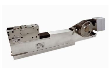
The ALF19-XS is typically used as central part in traceability solutions. It can be integrated in machines that place components on assemblies. In electronic manufacturing they allow a robust process applying uniquely serialised labels to products for traceability purposes, specifically where machine-readable bar code labels are used. With a full-automatic liner rewinding unit, the ALF19-XS also auto-collects empty label liners to keep the workplace clean.
