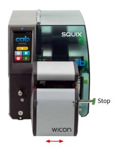
Label margins can be set 25 mm to 100 mm distant to the edge of an item using the stop.
